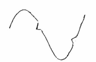
Waveform sides clipped at 180° by pulsating current flow. Average responding meters read too high. Only a meter that reads peaks at 180° can read correctly.
